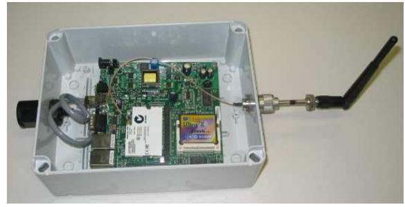
Fig. 3. Mesh Router with RB532a SBC and CM9 Wireless Card
