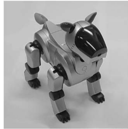
Fig. 2 One of the Sony Aibo ERS-210 robots used in the experiments. Note that the artificial auricles are mounted separately from the microphones (the three horizontal slits)
