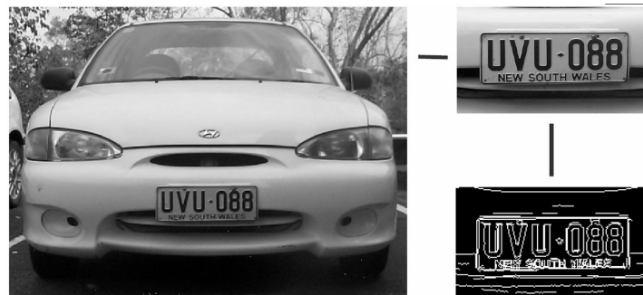
Figure 2. Dual-Resolution Camera with embedded edge detection
