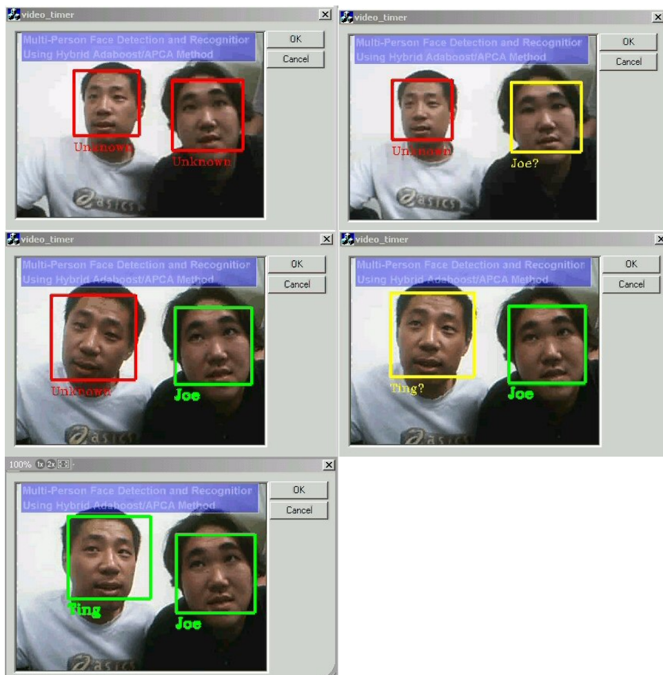
Fig. 5: Some selected frames (from left to right, up to down) showing different recognition confidence levels using different colour rectangles.
