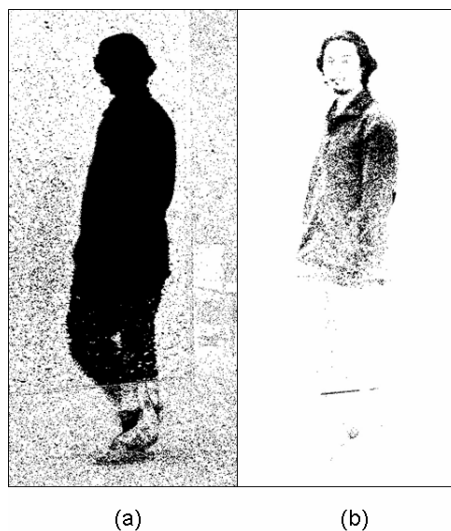
Figure 5: Background Subtraction using Low Threshold Value (a) and High Threshold Value (b)
