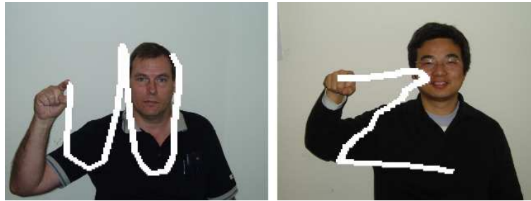
Fig. 3. “Fingerwriting:” Single stroke video gesture for letters “W” and “Z.”
